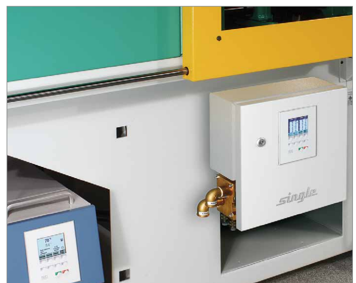
The SWV water distribution system used for flow metering in injection moulding machines
